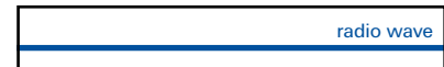
Cancellation of the radio wave due to an interference wave = flat line
